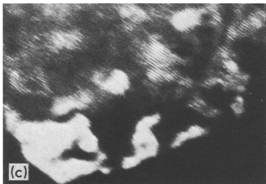
Figure 4 Surface topographical features of a \delta -FeO(OH) plate in (a) bright-field axial illumination, (b) and (c) tilted beam dark-field images from different reciprocal space regions.
